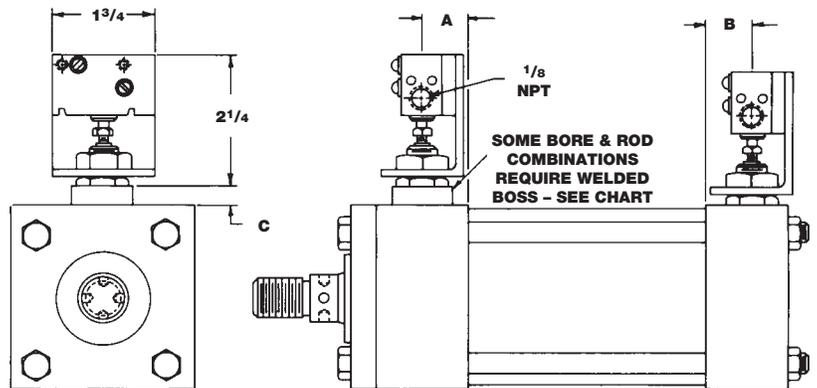
Switches are also available installed in the cap face as shown by **Illustration A**.
